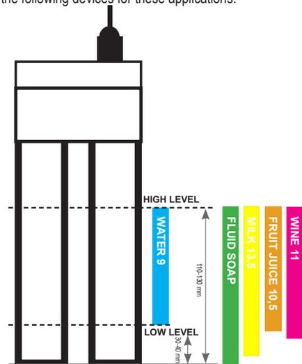
**Application:** Particularly suitable when there is not enough space for the movement of a traditional floating
