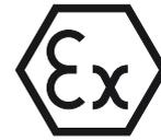
CE 0496 Ex II 2GD Ex db k c IIB T4 Ex tb IIIC T135°C IP68
